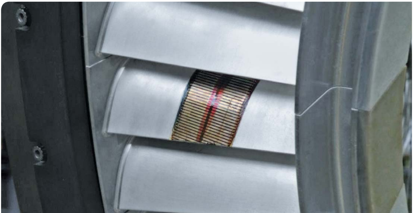
Turbine vane with hot film array for boundary layer investigations.
