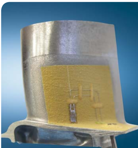
Turbine rotor blade with strain gauge (max. temp. 1,400 K).
