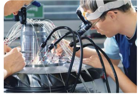
Instrumentation of a compressor rotor.
